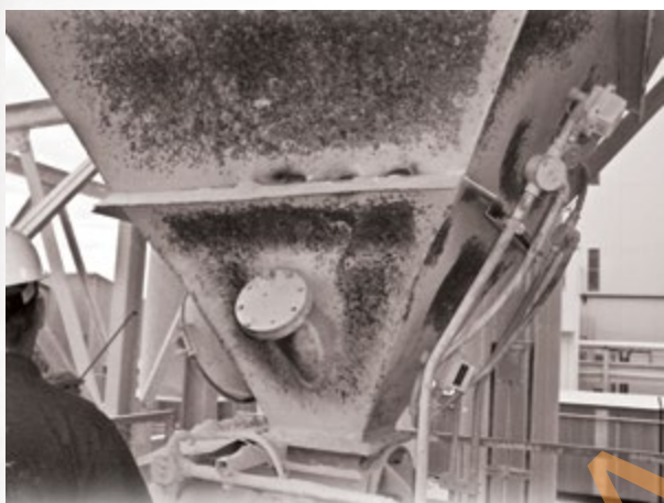
Hammering on the bin or chute wall leads to damage to the wall surface, often called "hammer rash."
